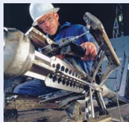
Engineer performs operational checks on the OBMI tool before a job.
