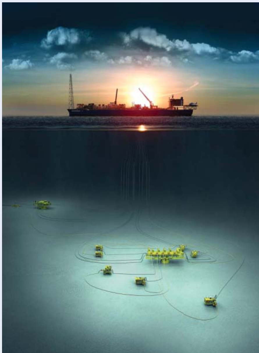
Dhirubhai I FPSO is positioned over the MA D6 subsea production system. The suezmax tanker was converted to a Aker's Smart FPSO with a processing capacity of 9 million cubic meters of gas and 60,000 barrels of oil per day.
